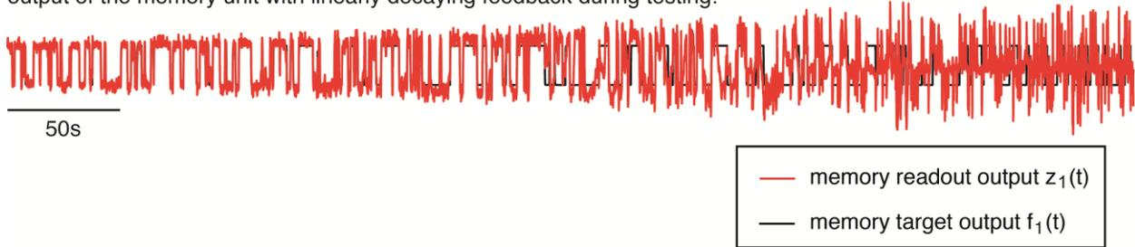
**Supplementary Figure S6:** Output of the memory unit in the switchable routing task with feedback weights linearly decaying to zero after learning. While the system is able to keep the memory states stable for a surprisingly long time despite the decaying feedback, the amplitude of the output is amplified rather than reduced, indicating a regulatory role of the feedback from the memory readout.
