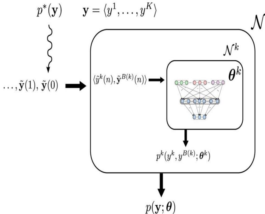
The network consists of 3-layer moduls, that each learn the probability table for one RV, conditioned on the RVs in its Markov blanket:
