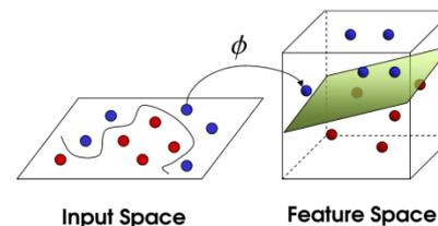
**Example:** *If a circuit precomputes all products  $x_i \cdot x_j$  of  $n$  input variables  $x_1, \dots, x_n$ , then a subsequent linear readout can compute any quadratic function of the original input variables  $x_1, \dots, x_n$ .*
