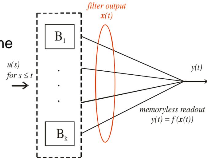
**Def:** A class  $\mathbf{B}$  of basis filters has the **pointwise separation property** if there exists for any two input functions  $u(\bullet), v(\bullet)$  with  $u(s) \neq v(s)$  for some  $s \leq t$  a basis filter  $B \in \mathbf{B}$  with  $(Bu)(t) \neq (Bv)(t)$ .
