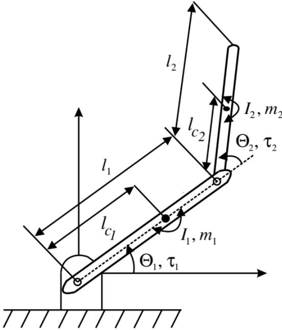
Figure 3: Standard model of a two-joint robot arm.
