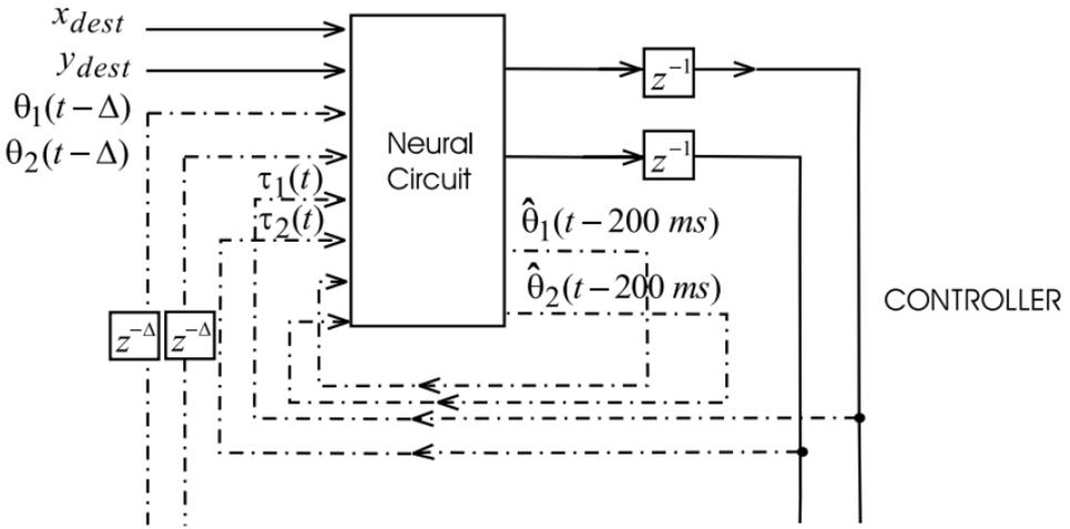
Figure 9: Information flow for the case of autonomously generated estimates  $\hat{\theta}(t - 200\text{ ms})$  of delayed feedback  $\theta(t - 200\text{ ms})$ . The rest of the circuit is as in Figure 2.
