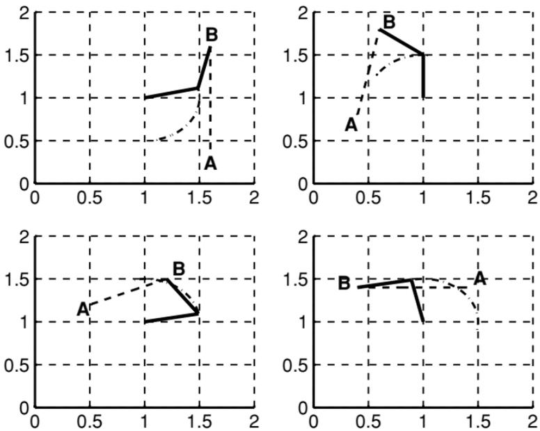
Figure 4: Initial position A and end position B of the robot arm (model 1) for four target movements, scaled in meters. The target trajectory of the tip of the robot arm and of the elbow are indicated by dashed and dashed-dotted lines. One sees clearly that even simple linear movements of the tip to the arm require quite nonlinear movements of the elbow.
